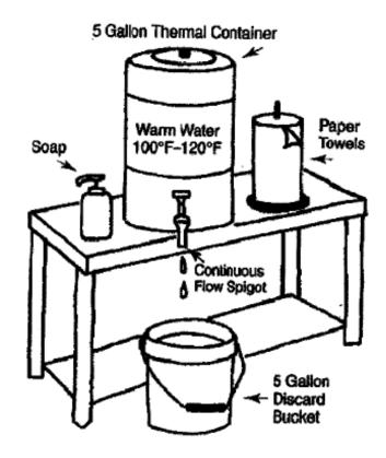
The temporary hand washing station shall consist of at least a 5-gallon insulated container with spigot that provides a continuous flow of warm (100°F- 120°F) running water, soap, paper towels, reminder sign, and a 5-gallon bucket to collect the dirty water.
